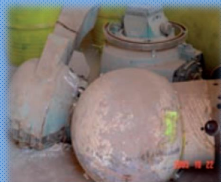
FIG. 14. Old ^{60}\text{Co} teletherapy heads.
