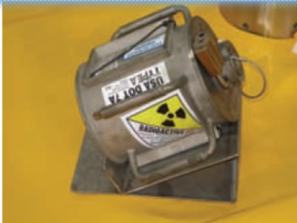
FIG. 35. Typical ^{137}\text{Cs} oil well logging source carrying shield (transport container). 37 kg × 170 mm diameter × 210 mm length (photograph: Schlumberger).
