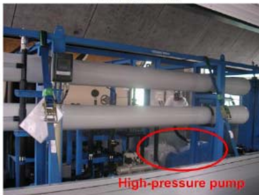
Reverse osmosis membrane in reverse osmosis membrane unit
